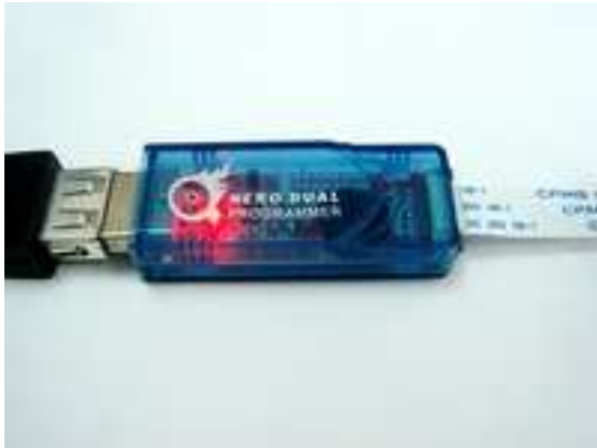
When it connect to PC USB and link success then RED LED will turn on
